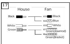
For pul chain controls, follow diagram above. Make sure that all exposed wiring is secured inside wire nuts. Note: Wires from house may vary in color and may not include ground wire. After wiring is complete, gently push wires into junction box with wire nuts pointing upward. Refer to point 3 of safety tips.
